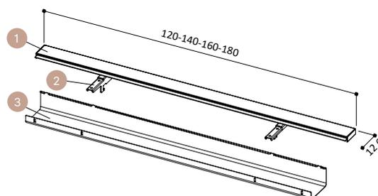
Fixing brackets with full length flap and cable tray for single desks
