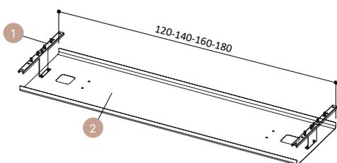
Fixing brackets with high capacity cable tray for bench desks with 38mm middle gap
