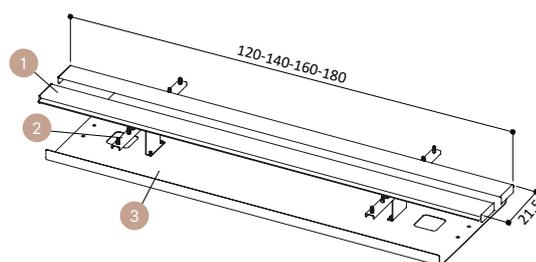
Fixing brackets with two full length flaps and high capacity cable tray for bench desks with 215mm middle gap
