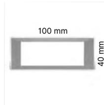
Beams made from 100x40mm rectangular 1.5mm epoxy powder coated steel tube.
