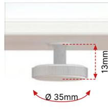
Loop leg frame: 0-13mm adjustable levelling feet made of polyethylene, 35mm diameter.
