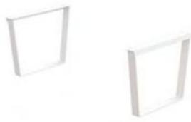
Loop legs made of 50x6mm epoxy powder coated steel flat bar welded to two 3mm thick steel mounting plates. Supplied with antislip felt pads.
