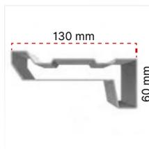
Perimeter frame made from 1,5m steel tube, 130x60mm section.
