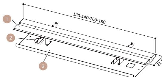
Fixing brackets with two full length flaps and high capacity cable tray for bench desks with 215mm middle gap
