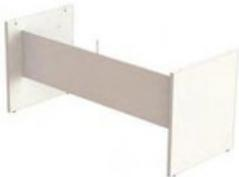
Panel legs made of 25mm melamine faced chipboard (MFC) with 2mm matching impact resistant Abs straight edges. 18mm Mfc structural modesty panel with matching melamine straight edges. Easy to clean scratch-resistant anti-reflective melamine
