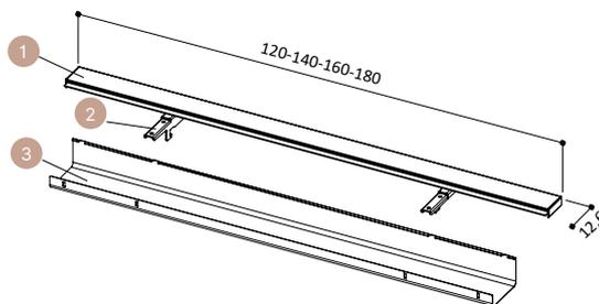
Fixing brackets when no cable management is required
